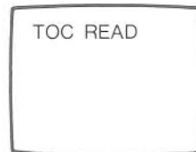
Reading the content of the disc. ●This Display will be indicated when a CDV or CD disc is inserted.
